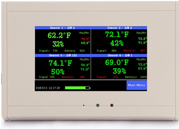
It is the only instrument that monitors, alarms, logs and charts temperature and humidity as a stand-alone device. Although it is a very sophisticated electronic instrument it has a simple user interface. It has a color Easy Touch display which responds to a finger tip touch.
