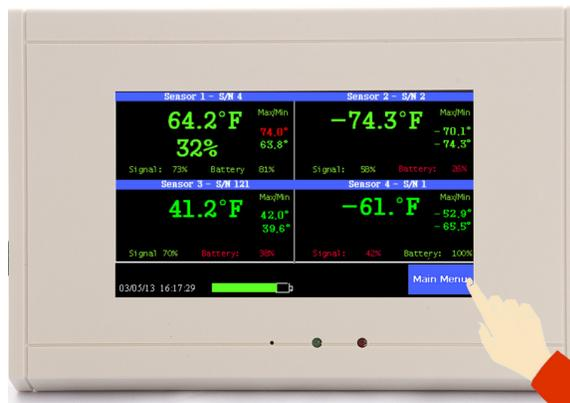
The Master Thermometer is being used extensively to monitor refrigerators and freezer where vaccines and medicine are stored. It has an internal alarm which sounds a high pitched alarm and flashes the screen when an alarm is triggered. It also has a relay so that external alarms, sirens, or lights can be triggered upon alarm. Many Master Thermometer users are installing an auto dialer so that a phone call is triggered if the temperature gets too warm or cold for too long.
